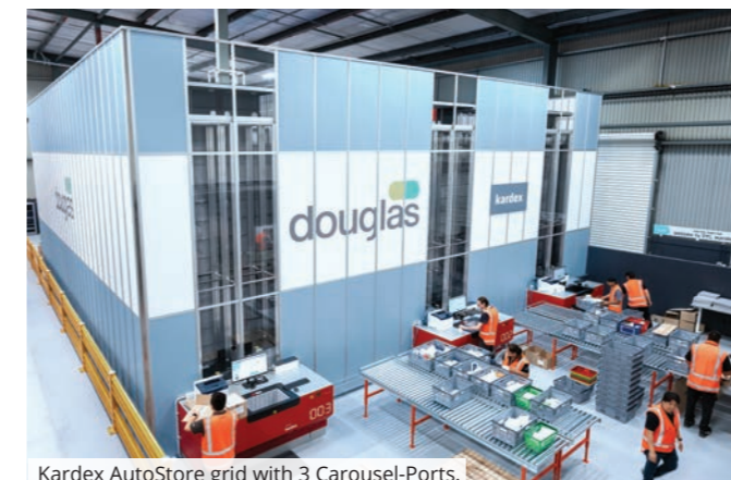
Kardex AutoStore grid with 3 Carousel-Ports.
